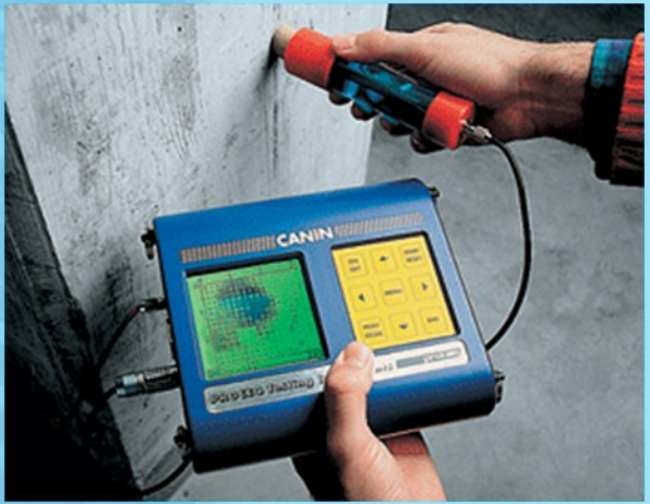
Corrosion Analyzing Instrument
