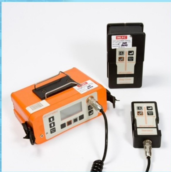
Bar Locator And Cover Depth Meter
